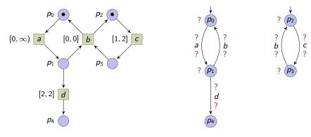
Add one clock to each automaton. The clock is reset on each edge.
