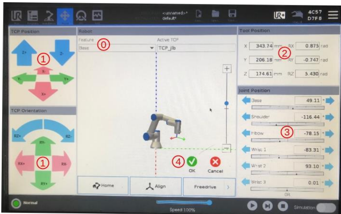
Figure 12: Setting point Waypoint_1 .
